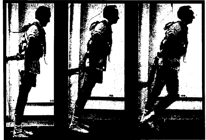
Figure 1. Computer-assembled subject configurations during the initial stages of the response. Left: Before release. Center: Shortly after release. Right: At approximately the time of right foot liftoff. The horizontal belt attached to the lean-control cable is behind the subject, at waist level. The vertical safety harness support cable, some of the infrared-emitting diode markers, and portions of the forceplates can be seen.
